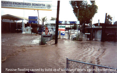
Nassive flooding caused by build up of windswept debris against border fence
